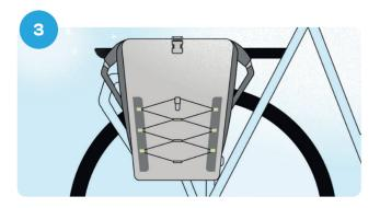
Snap your MIK side bag onto this system of three (pre-installed or included) Studs.
